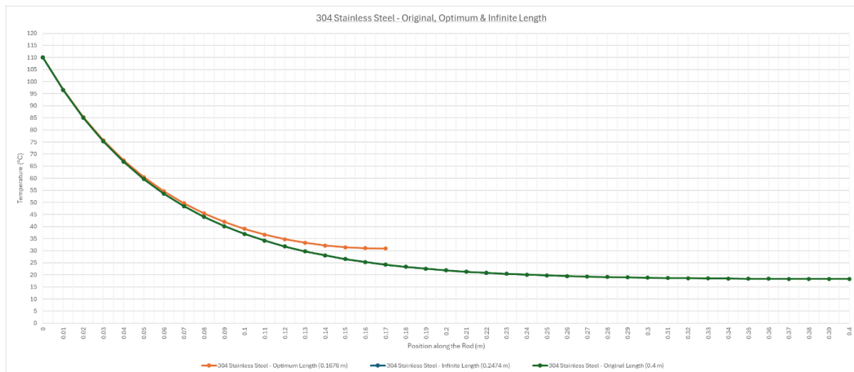
Figure 10: 304 Stainless Steel - Original, Optimum and Infinite Temperature Distribution.
