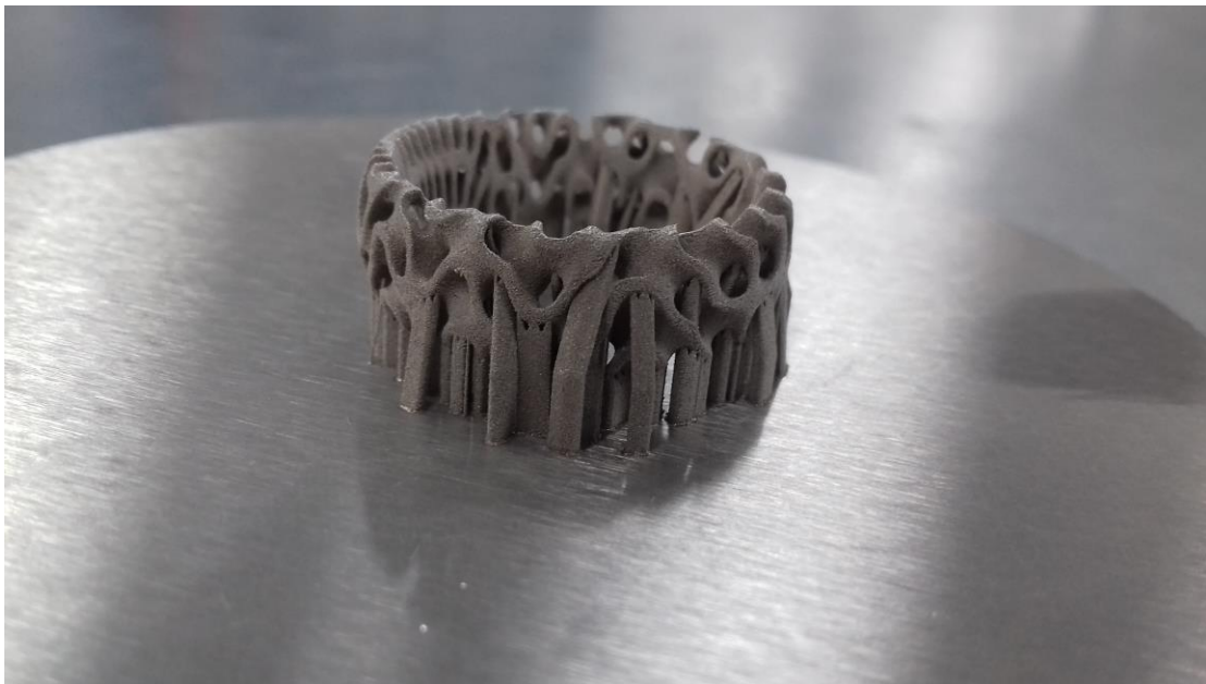
Figure 55: Finished ring with support structures (Watts & Hill, 2022.)
