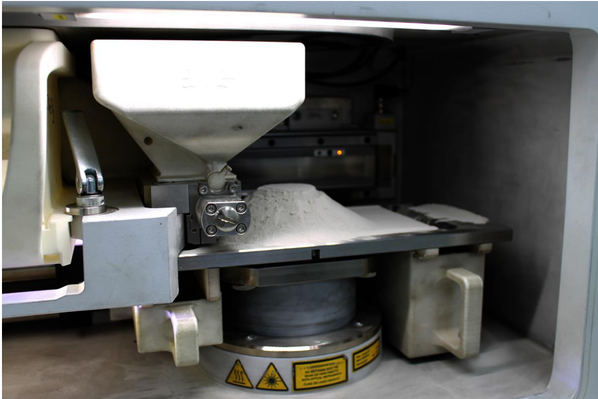
Figure 24: Isla Cocos SLM build at Cooksongold EOS M-80 (Watts & Hill, 2021).
