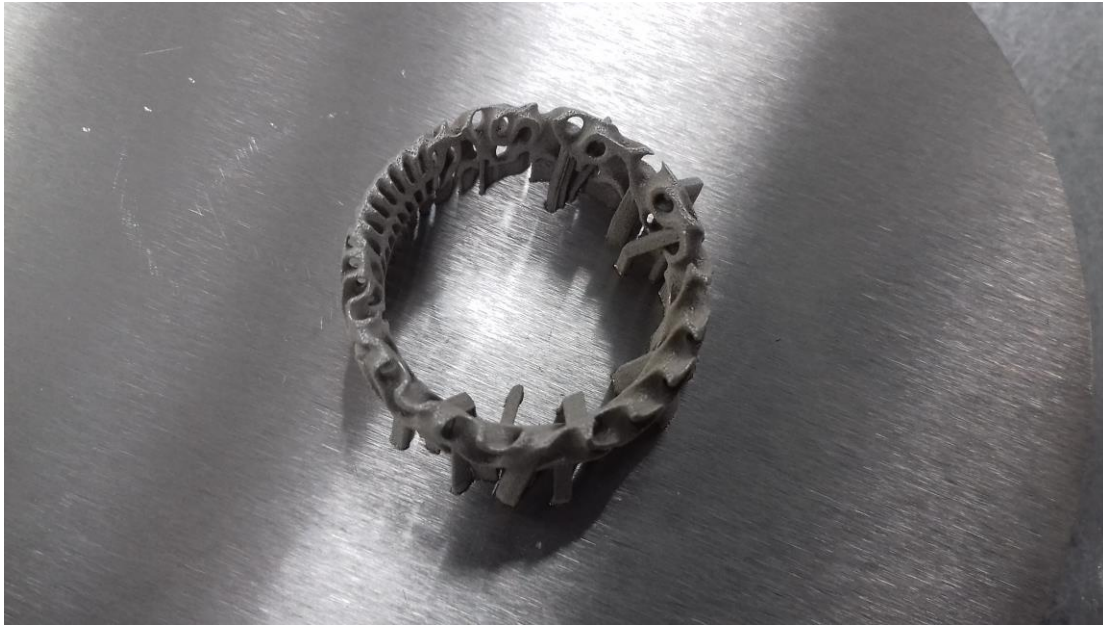
Figure 56: Finished ring top view with support structures (Watts & Hill, 2022.)
