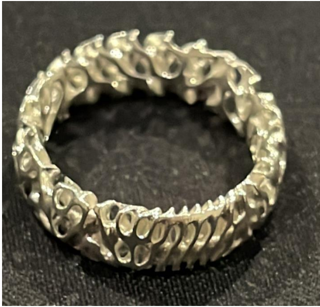
Figure 46: Silver Sample support removal, post production with 800 & 1200 grit paper, magnetic polishing & hand Polishing with polishing compound (Evans, 2023.)
