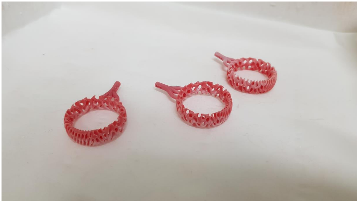
Figure 43: Red MJP wax builds of TPMS Diamond ring (Gucci, 2022.)
