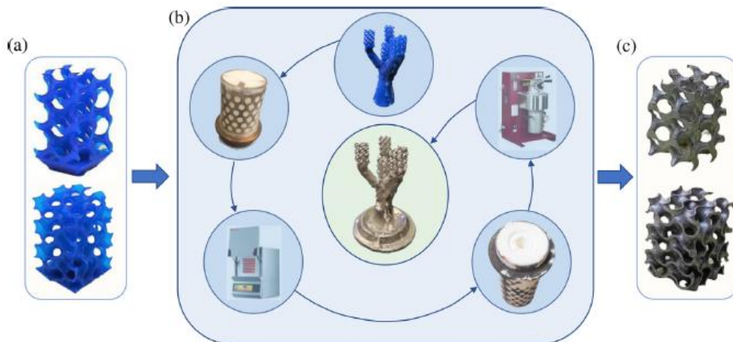
Figure 4: Lost wax investment casting stages of TPMS constructs (Al-Ketan, Singh & Karathanasopoulos, 2023).
