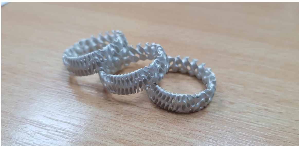
Figure 45: Silver samples post cast, & removal from tree with wire cutters (Gucci, 2022.)
