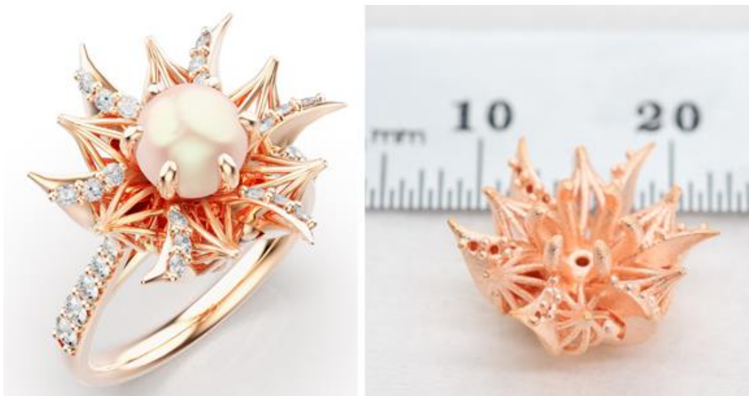
Figure 28: Keyshot Render of Holo ring & subsequent pure copper trial part (Metal Additive Manufacturing, 2021).
