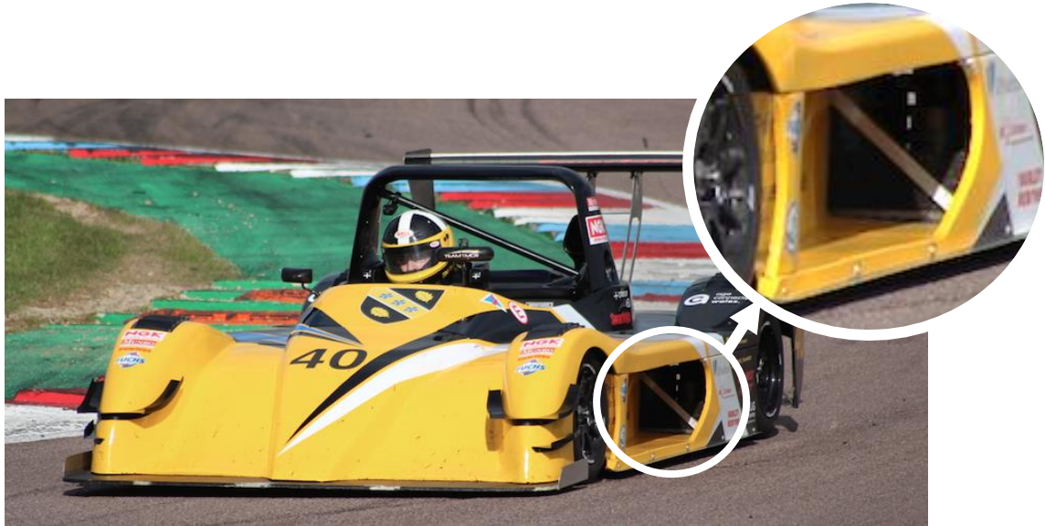
Figure 3-10 proposed KERS radiator location (M Sport Eng, 2016)
