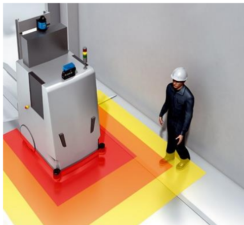
Figure 7 - Illustration of Proximity Detection (Pastor, 2022)
