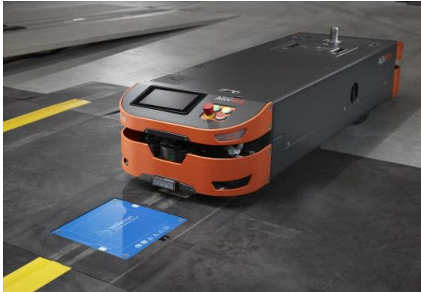
Figure 6 - Wireless AGV and AMR charging (Wiferion, 2023)
