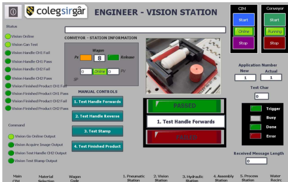
Figure 17 Engineers vision station HMI
