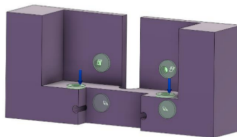
Figure 2 Boattail Constraints and Loads
