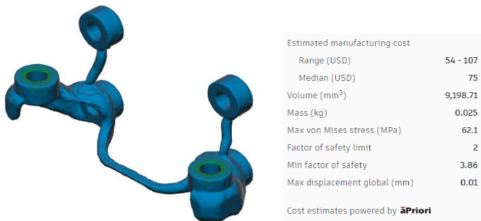
Figure 10 Generative Design of Boattail
