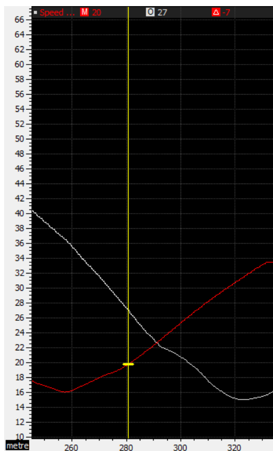
Figure 7: Speed (m/s) vs. Distance (m) at Corner 1 for two spring rates
