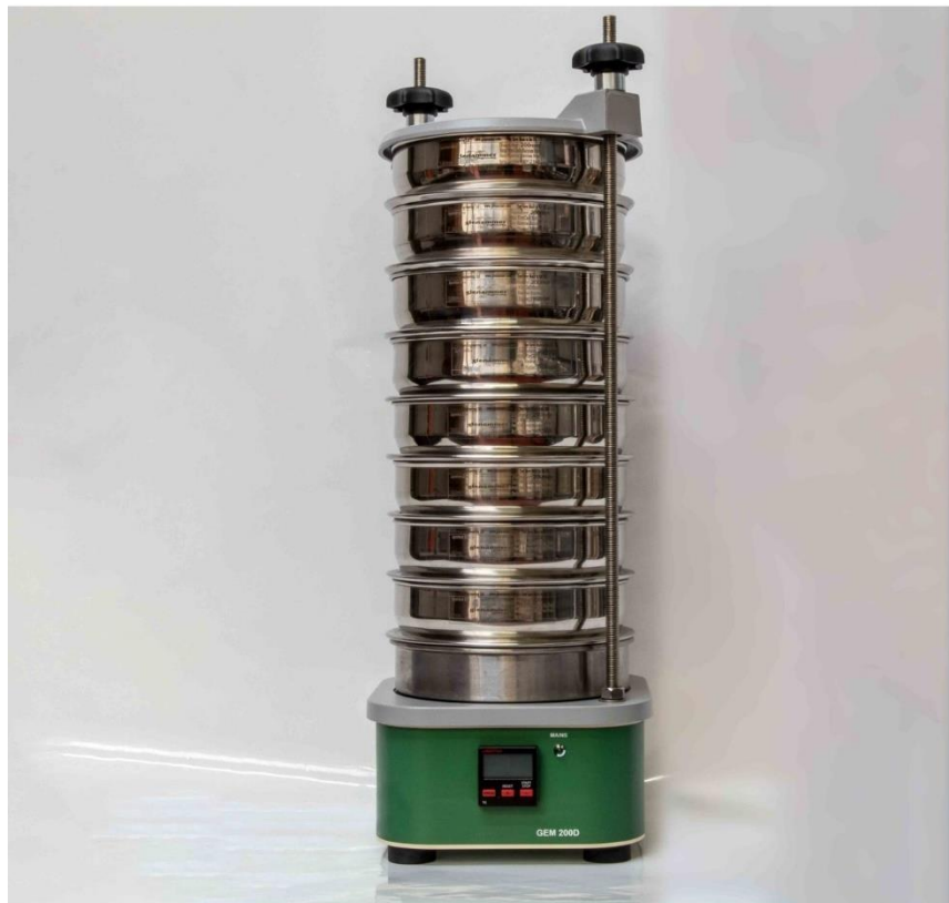
Figure 4. Sediment sieve stack.
