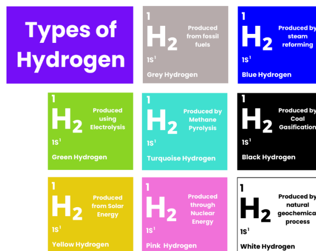
Figure 16: Hydrogen Colour Spectrum (Examples, n.d)
