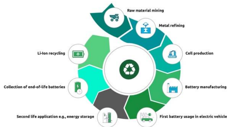
Figure 22: Lithium-Ion Battery Life Cycle (Tschödrich, et al., 2022)
