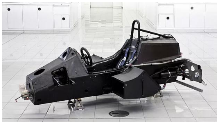
Figure 2 – McLaren Carbon Fibre Monocoque (Motorsport, 2022)
