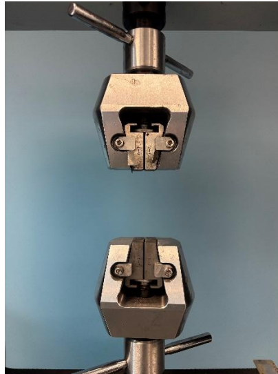
Figure 6 - Denison Machine wedge-action grips
