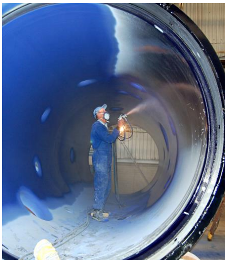
Fig 8. Manual spray application of enamel coat (The Vitreous Enamellers Society, 2019)
