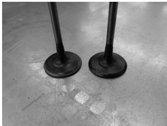
Figure 48 - Lapped valve compared to the original acquired valve.
