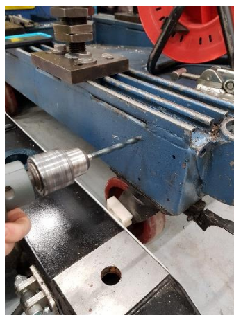
Figure 3-49 - Drilling Holes for Clamps
