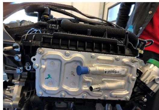
Figure 35 - CAC integrated into the intake manifold
