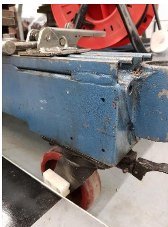
Figure 3-48 - Holes Drilled for Clamps
