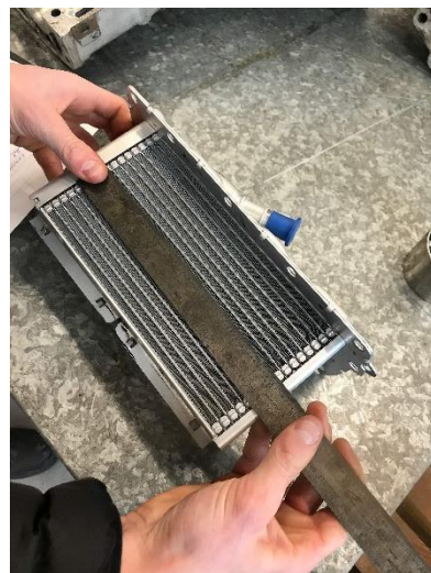
Figure 33 - Measuring the CAC for the CAD model
