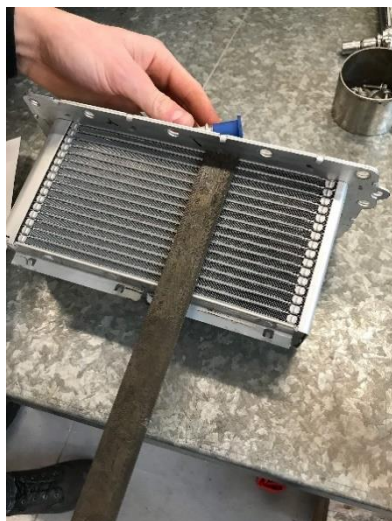
Figure 32 - Measuring the CAC for the CAD model
