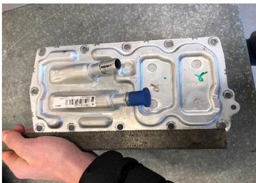
Figure 34 - Measuring the CAC for the CAD model
