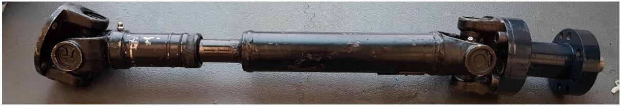
Figure 3-43 - Cardan Shaft Bolted to the Painted Adapter Shaft
