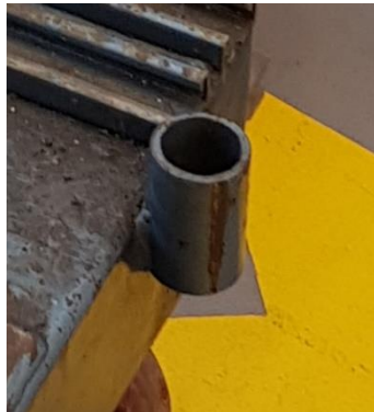
Figure 3-44 - Random Cylinder Welded to Trolley That Was Removed
