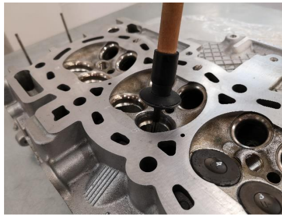
Figure 47 - Image showing the lapping process of cylinder.
