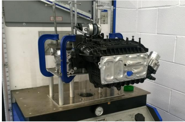
Figure 52 - Complete intake manifold system with an inbuilt charge cooler mounted on the flow bench.
