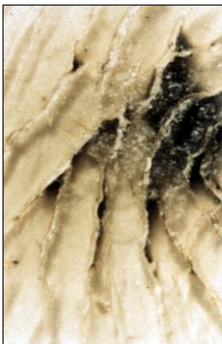
Figure 5-11 Shear bands seen on thermally sensitive paper recovered from a drop-weight impact on HMX sample (Courtesy of Imperial College London)
