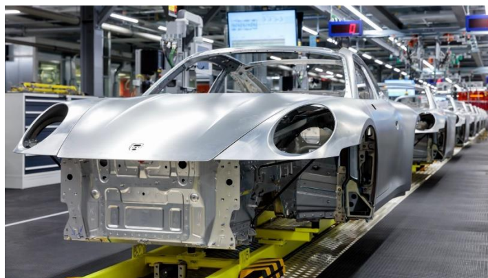
Figure 2 - Porsche's new production line for the 992 generation, showing automation has become a main part of production lines.
