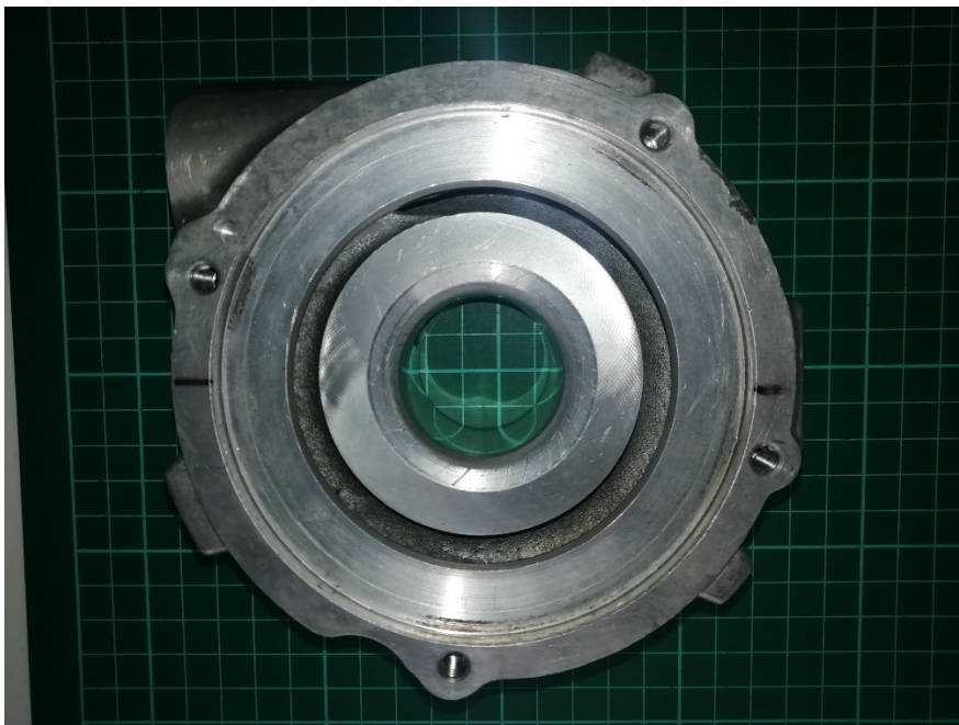
Figure 12, inside view of real compressor housing.
