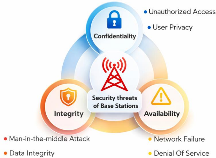
Figure 2. Security Threat Of Base Station
