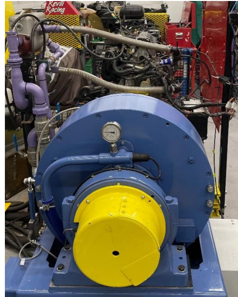
Figure 2. Honda CRX engine mounted on the ECD (Aganon, 2023)
