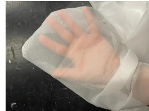
The other synthetic fabric I experimented with; I found it was too thin and the shine on the material made it so you can see a halo around the beam projected at it.
