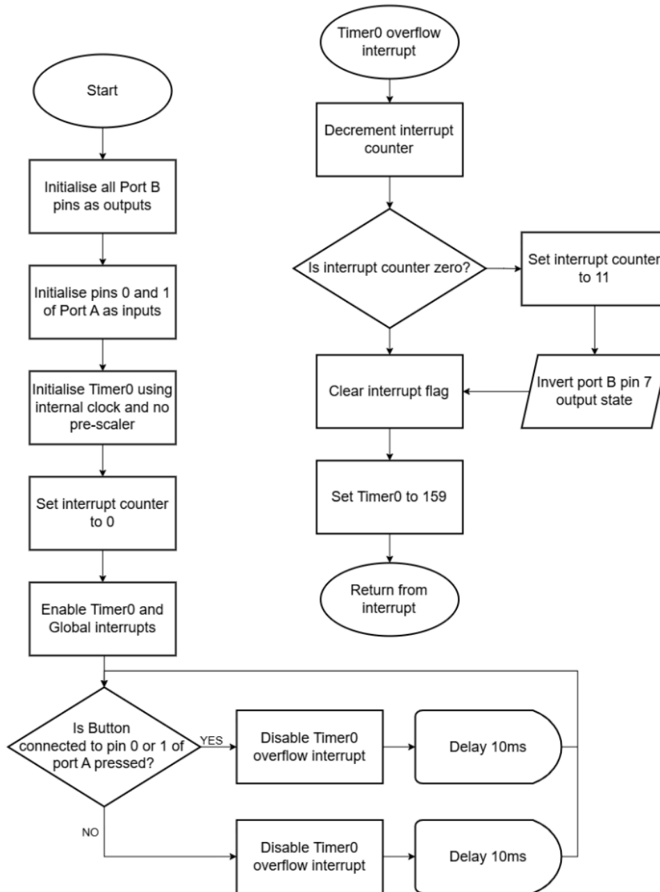
Figure 18. Flowchart illustrating the logical operation of the Sounding the Piezo Buzzer PIC assembly code.
