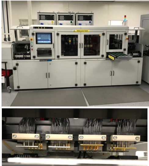
Figure 13: Electrical Test Machine (top) and Internal contact points (bottom) (Source: KSR & Thomas, 2017)
