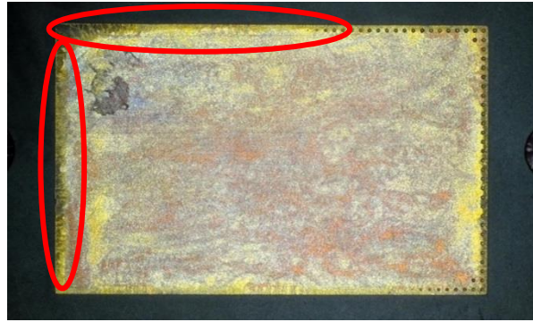
Figure 5: DBC with missing dimples (Source: KSR and Thomas, 2017)
