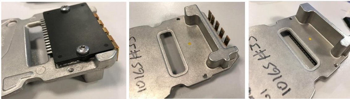
Figure 8: Power Module attached to customer's heatsink (Source: Thomas and KSR, 2018)
