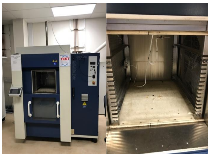
Figure 10: Thermal Shock Chamber (Source: KSR and Thomas, 2017)
