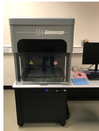
Figure 12: CSAM ultrasound (Source: KSR and Thomas, 2017)
