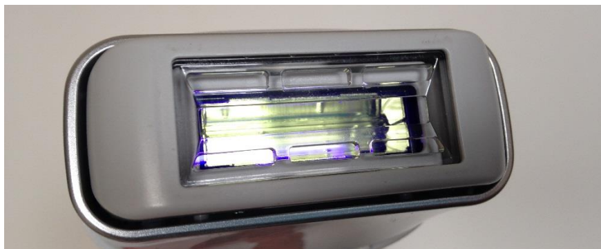
Figure 5.2 - Device 6 only had a large mechanical push switch to activate the flashes. This could easily be overridden when not in contact with the skin by manually pushing on the switch.
