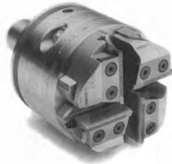
Fig. 3E4 A die head for external threads with inserted multi-toothed cutters. (Courtesy Landis Threading Systems.)
