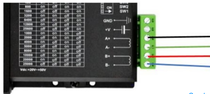
Figure 17, Motor connection.
