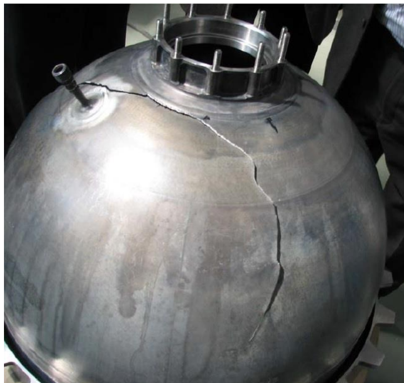
Fig. 4: Stress-corrosion Cracking in Titanium Propellant Tank for Vega Rocket (The European Space Agency, 2014)
