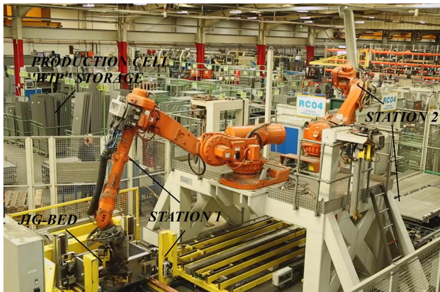
Figure 1 RC04 Robot Welding Cell Image (Bisley, 2018)
