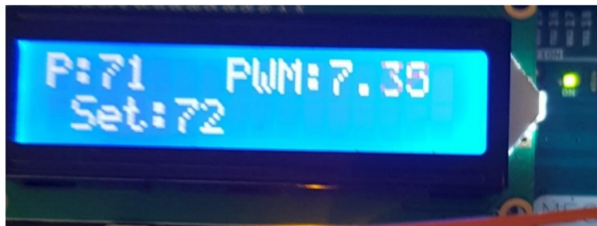
Figure 61 - Pressure close to set point PWM slowing down
