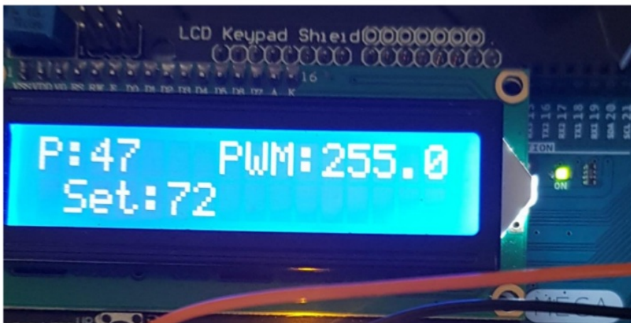
Figure 64 - Pressure exceptionally low below set point PWM asking for full 255 demand
