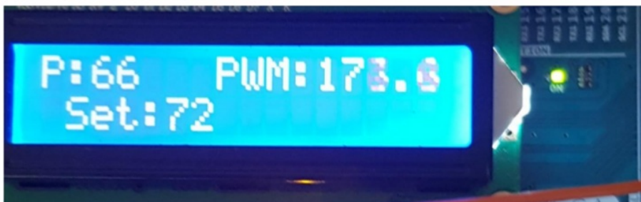
Figure 62 - Pressure below set point PWM demand increased
