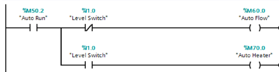
Figure 15 - Automatic Control (Network 1 & 2)
