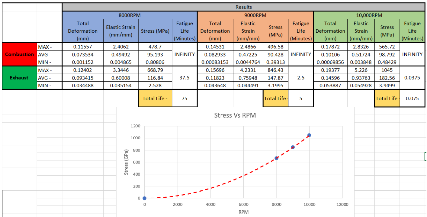
Figure 9 – Results from Ansys connecting rod study
