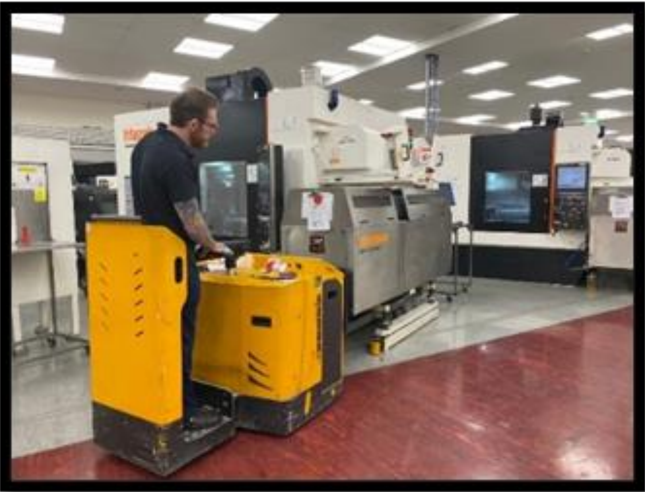
RAMTIC Carousel being loaded onto a MAZAK FJV using a roller truck.
