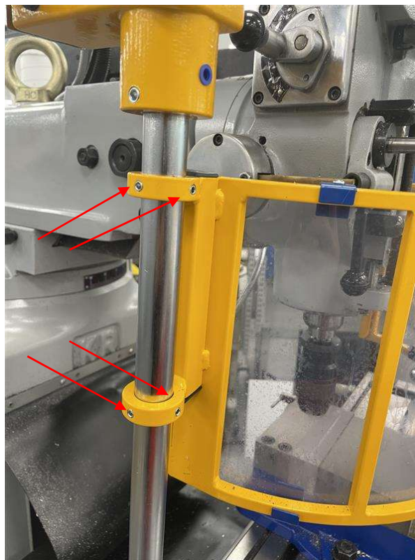
Figure 30 - New spindle guard grub screws
