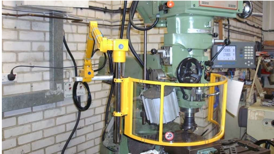
Figure 9 - Adjustable interlocked guard (PUWER Machinery Guarding, 2025a)
