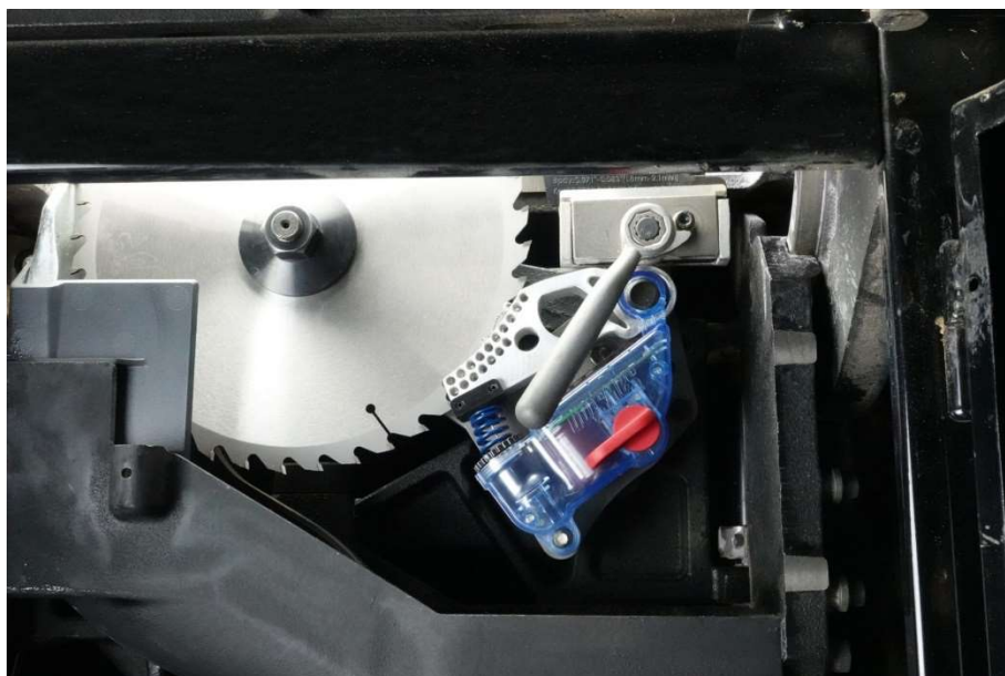
Figure 11 - SawStop Break Mechanism (SawStop, 2025)
