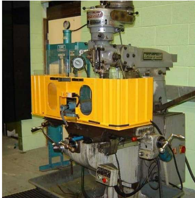
Figure 8 - Interlocked Milling Machine Guard (PUWER Machinery Guarding, 2025b)
