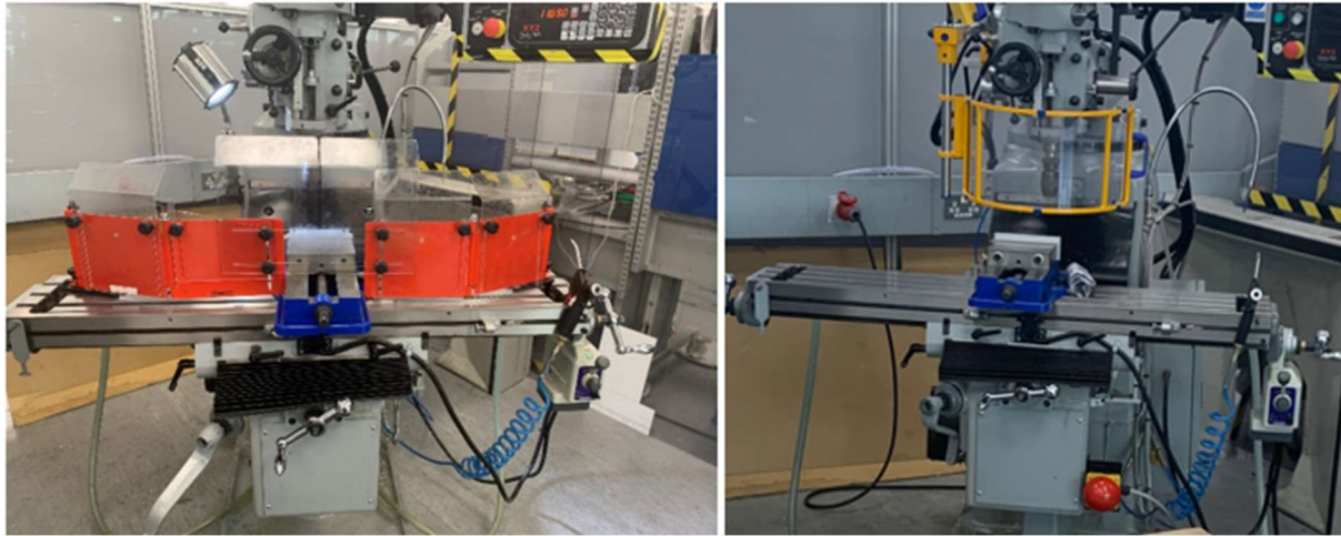
Figure 32 - Old Guard (left) vs New Guard (right) Vice Test
