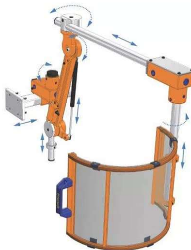
Figure 21 - Adjustable interlocked milling machine guard
