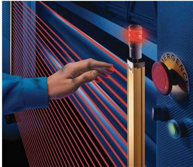
Figure 14 - Light Curtains (Association for Advanced Automation, 2024)
