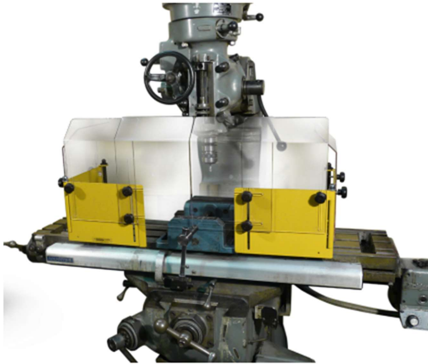
Figure 6 - Fixed Milling Machine Guard (Silvaflame-Cleervue, 2025)
