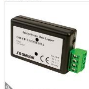
Figure 42: Cost Effective Data Logger (Omega, n.d.)
