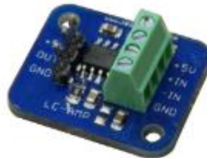
Figure 40: Suggested Amplifier (Leo Bodnar Electronics, n.d.)
