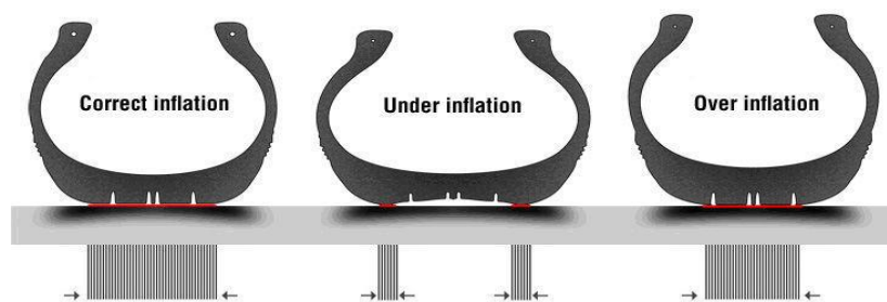
Figure 8: Inflation pressure versus Contact Patch (Tyre Leader, n.d.)
