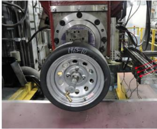
Figure 15: Rig used on Round 9 of FSAE TCC testing (FSAE Tire Test Consortium, 2022)
