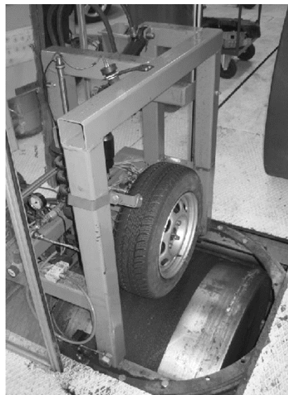
Figure 10: Tyre Testing Rig used for FE development (Korunović*, Trajanović, Stojković, Mišić, & Milovanović, 2011)
