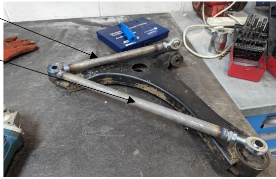
Figure 21: Completed Wishbone, compared against the original
