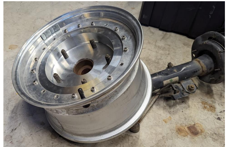
Figure 37: Wheel Adapter Fitted to Rim
