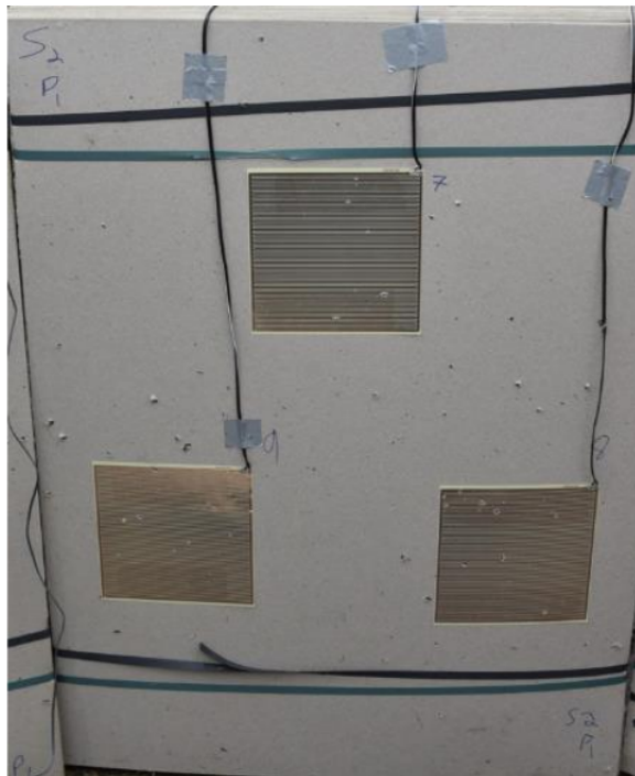
(Figure 2- Velocity Foils taped to strawboard)
