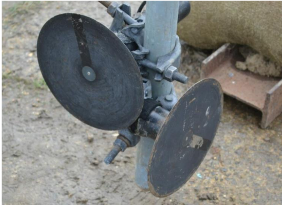
(Figure 3- Blast Pressure Gauge, Steel overcover, nylon bush covering pressure sensor in the centre)
