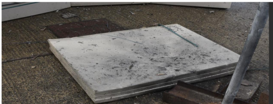
(Figure 3- Explosive residue left on test bed)
