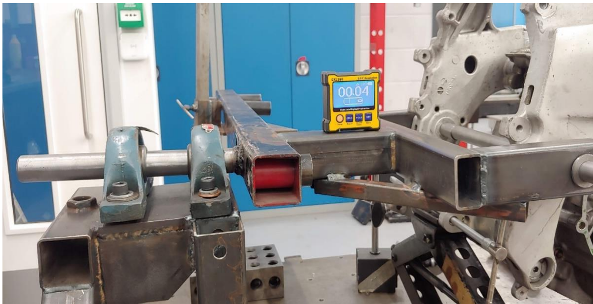
Figure 10 Horizontality check throughout digital inclinometer
