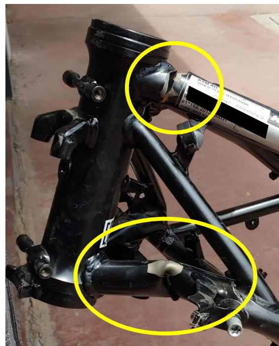
Figure 1 Chassis' failures example
