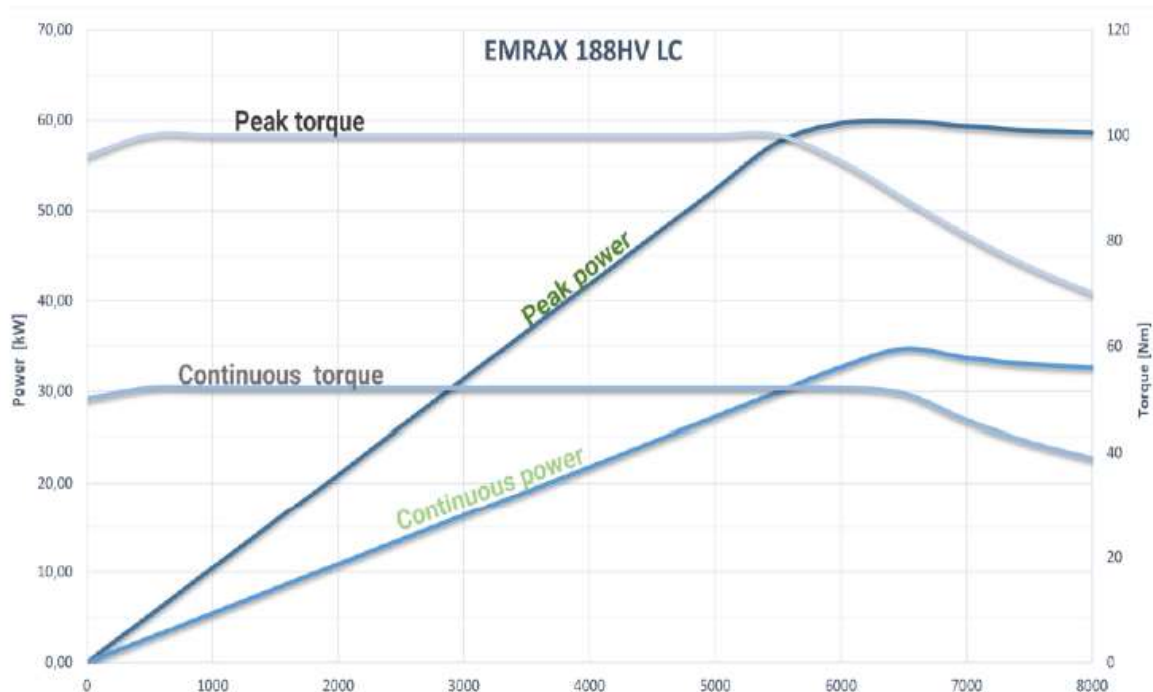
Figure 8: The Emrax torque profile. Continuous torque remains at about 50Nm for nearly the entire operating range of the unit, and may peak as high as 100 Nm for two minutes (Emrax 2023).
