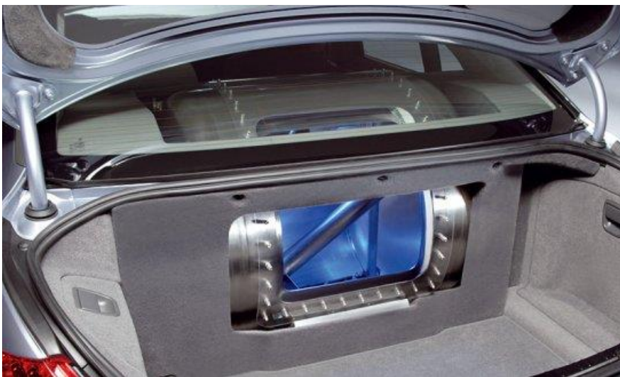
Figure 2 Cross section of liquid hydrogen fuel tank from BMW's Hydrogen 7
