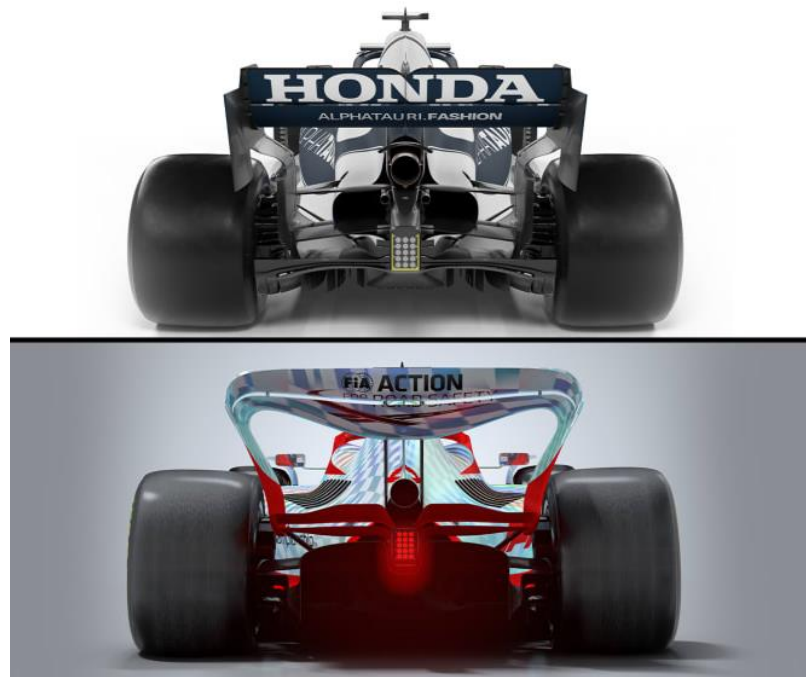
Figure 13 2021 Rear Wing vs 2022 Rear Wing (Reynolds, 2021)
