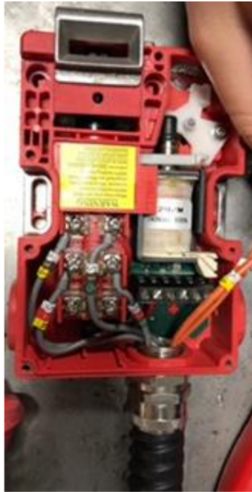
Figure 31 - GuardMaster Door Switch
