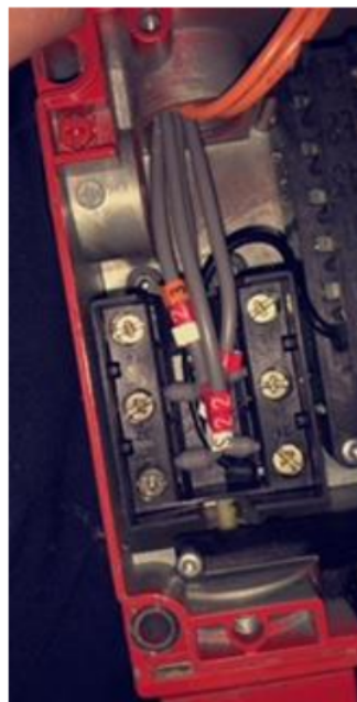
Figure 30 - GuardMaster Door Switch
