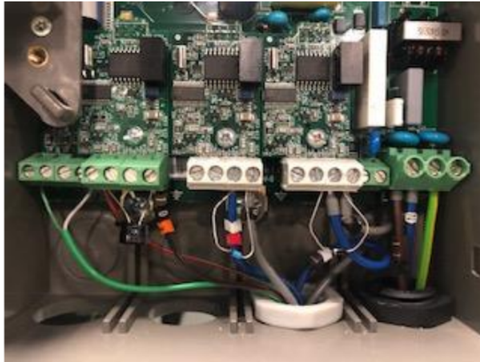
Figure 35 - Data Logger Connections
