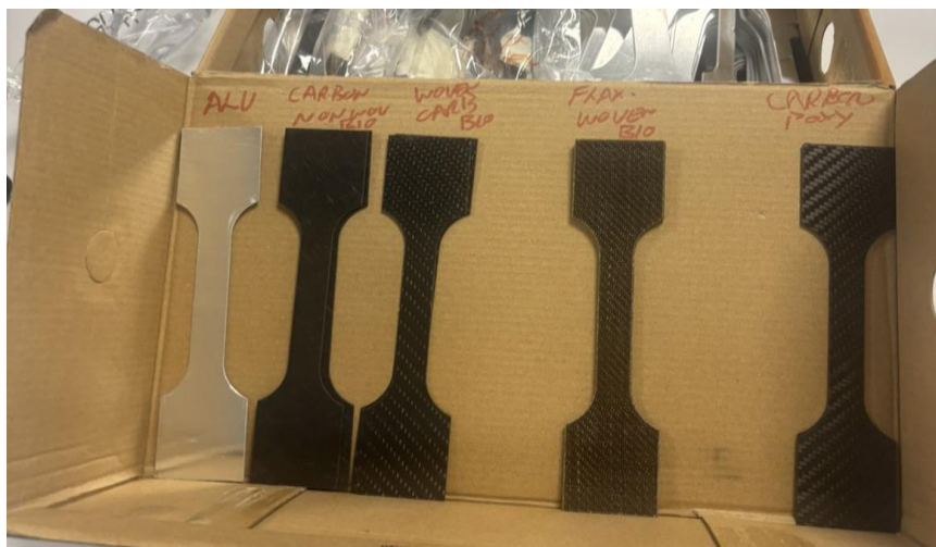
Figure 1 - Test Samples Before Fracture
