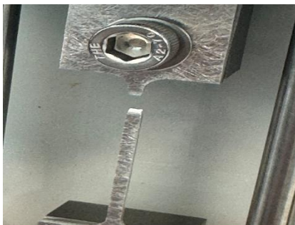
Figure 2 – Tensile testing – Specimen reaches Fracture by elongation
