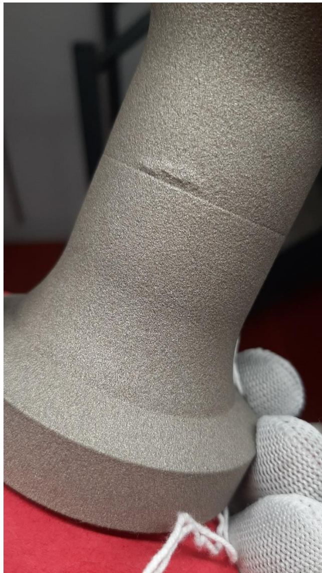
Figure 2: A blistered part that has been bond coated.
