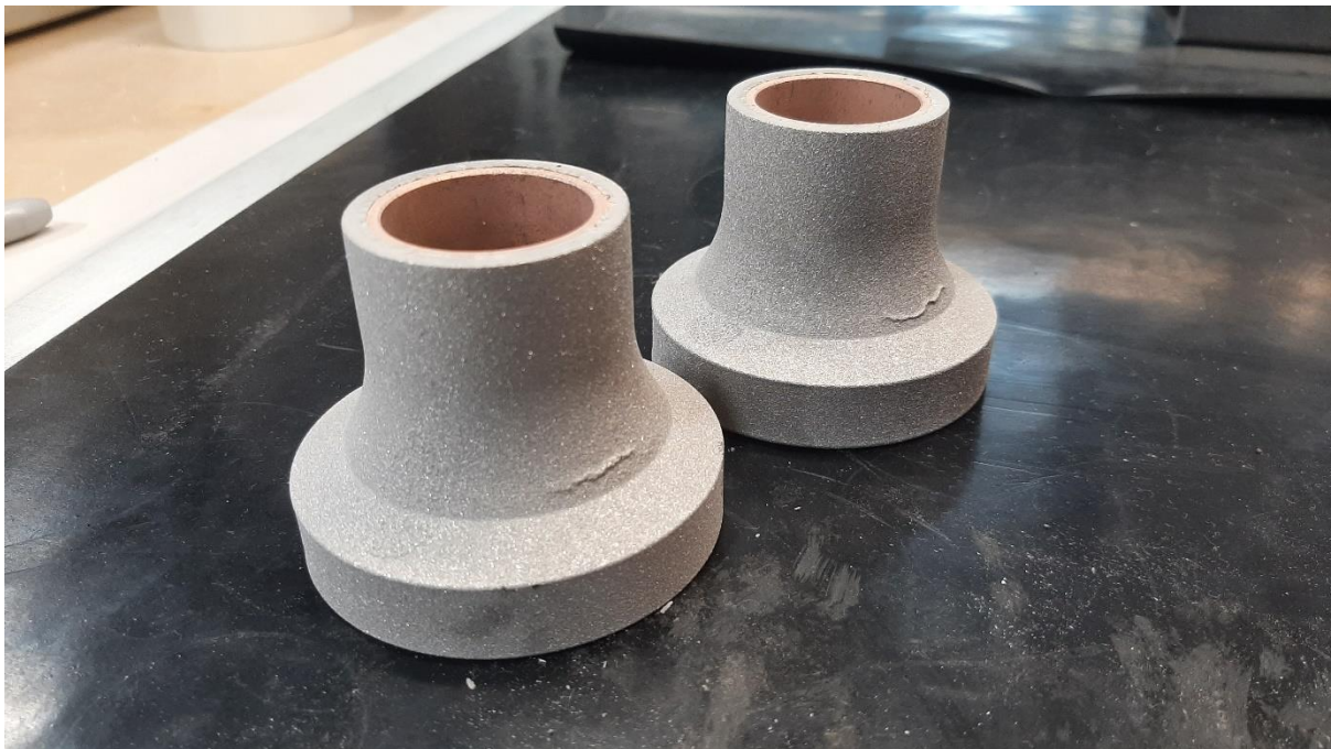
Figure 4: Minor Shoulder Blisters
