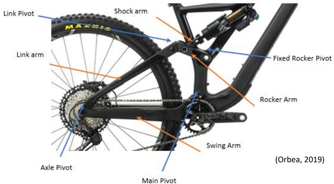
Figure 1 Orbea Rallon Linkage System Explained
