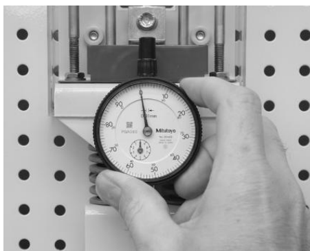
Figure 3: Setting the dial indicator to zero
