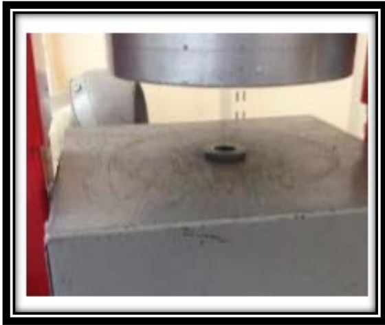
Figure 6: Picture of a Bellville washer being tested on a spring compression tester (Smith, Stanford & Cutlan, 2015)
