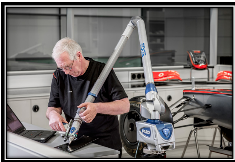
Figure 54: Picture of a faro arm being used for a formula one application ( www.faro.com , 2012)
