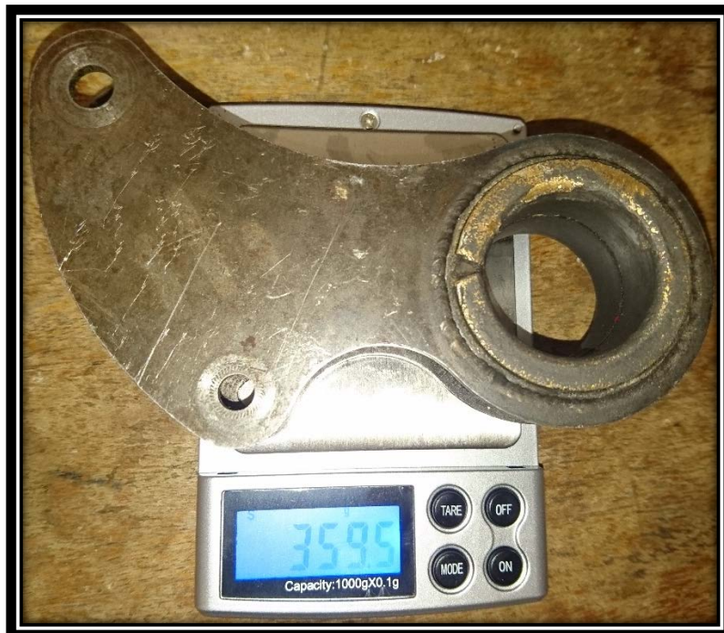
Figure 50: Picture showing RC97 bell crank being weighed.
