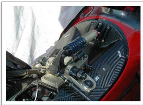
Figure 4: Picture showing mono-shock layout with centrally mounted damper. ( www.tezzaworld.com/ , 2015)
