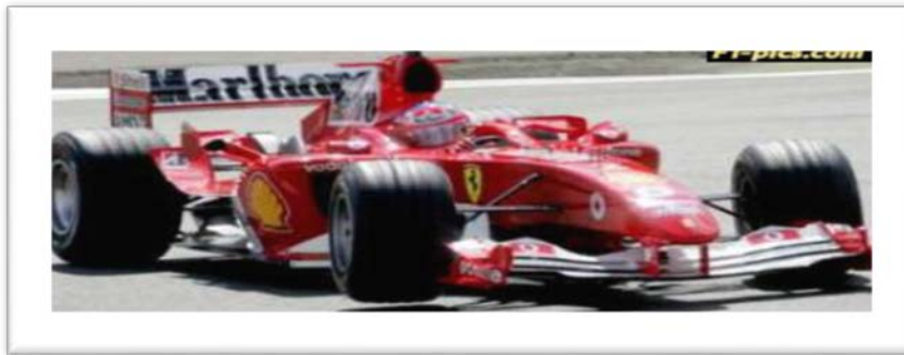
Figure 3: Picture showing a F1 car cornering with inside wheel lifted off the ground. (Dilworth, 2011)
