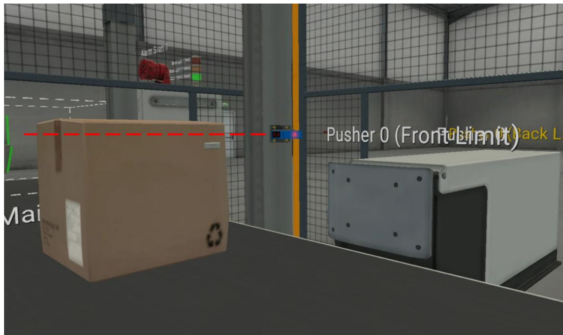
Figure 3: Large package diffuse sensor location.
