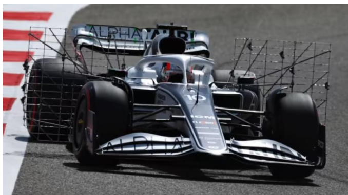
Figure 6: Aero rakes being used to collect airflow data. (Formula 1 , 2023)
