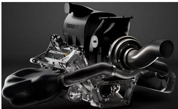
Figure 5:Hybrid Turbo V6 Engine (Josheph, 2014)
