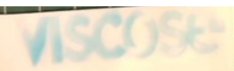
Figure 4: Blue ink print example after the washing process containing sodium chloride and sodium carbonate
