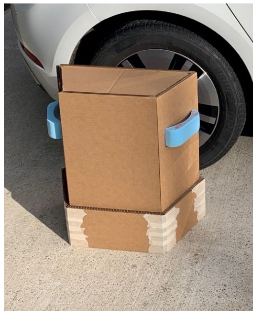
Figure 6 Full scale cardboard model with handles and kick shielding for testing.
