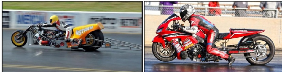
Figure 19 - Comparison of Rake Angle, with Wheelie Bars (Left) (Storm, 2013) and without Wheelie Bars (Right) (Dragbike.com, 2018)
