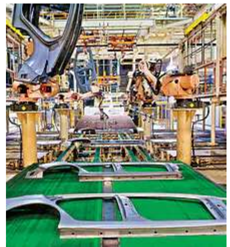
Robots with suction cups position body panels on inventory racks.
