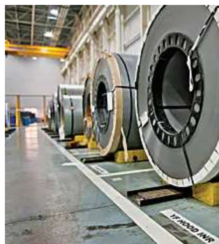
Coils of steel will be stamped and formed into doors, hoods, trunks, or side panels. Hyundai is the only automaker producing its own steel.
