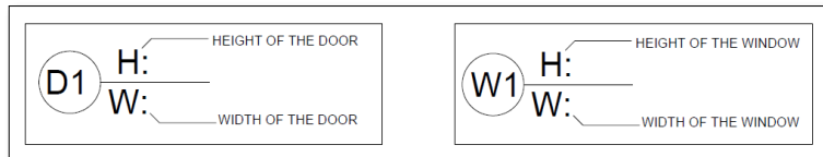
Fig.1.5. Window & Door Symbol in Plan
